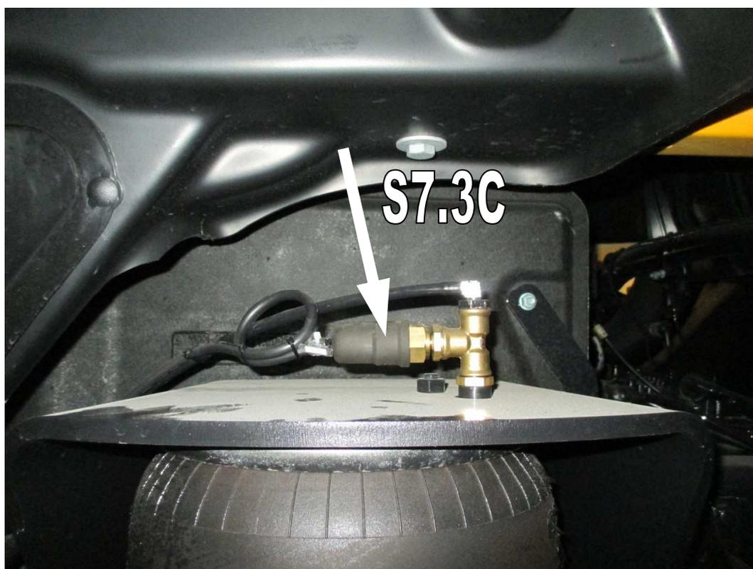
**Image 21 – pressostat essieu avant**
